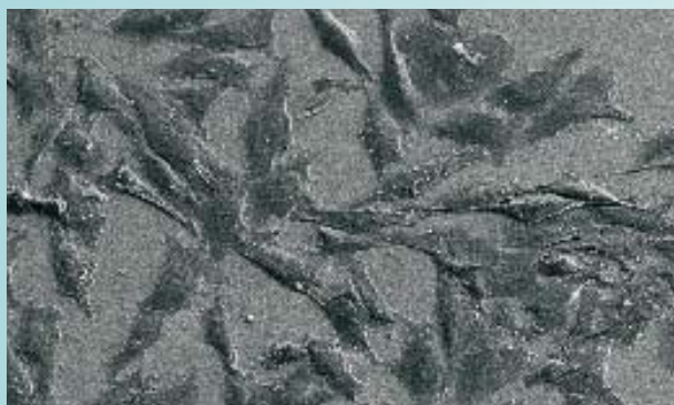
Figure 2. Electronic microscope image of the osteoblast culture on smooth titanium after 24 hours of incubation. Flat morphology of osteoblasts is observed.
