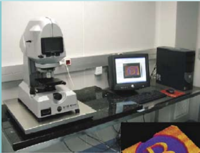
Figure 2. WYCO NT 1100 interferometer microscope
